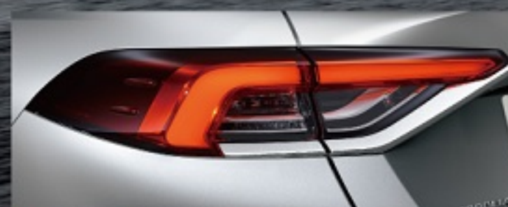
LED光條式尾燈 (HYBRID車型、GR SPORT車型、汽油尊爵+/尊爵)
