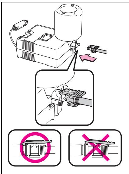
**5 從刺破輪胎的氣嘴上拆下氣嘴蓋。**
